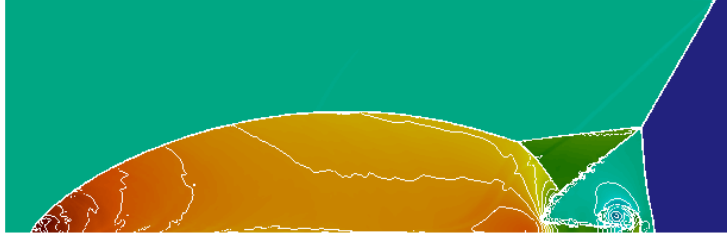
Figure 3: Double Mach reflection test case, polynomial order k = 2 , \Delta x = \Delta y = \frac{1}{360} , without shock indicator.
