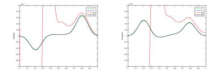
Figure 4: Perturbation of an equilibrium solution of amplitude  $A = 10^{-5}$  for well balanced schemes of order 3 and 5 (green and blue curves), and non well balanced schemes of order 3 and 5 (red and black curves). N = 40 points per unit length.
