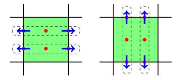
Figure 1: Illustration of the well-balanced quadrature rule for the source term in two space dimensions. Numerical fluxes are represented by the arrows, red dots represent the quadrature nodes for the source terms.
