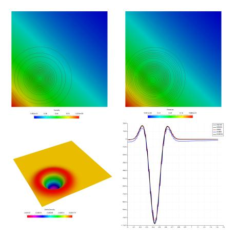
Figure 6: Top: density (left) and pressure (right). The contours represent the perturbations (20 isolines between -0.001 and 0.0002) for  $\rho$  and 20 isolines between -0.00027 and 0.00027 for p). Bottom left: extrusion of the density perturbation. Bottom right: comparison of the density for different grids and schemes (black lines for  $\Delta x = 1/100$  and  $\Delta x = 1/200$  balanced,  $\Delta x = 1/100$  WB; red for  $\Delta x = 1/50$  WB; blue for  $\Delta x = 1/50$  UNB)
