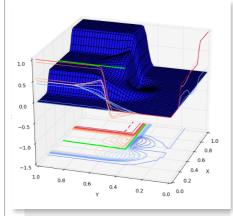
The numerical solution of the x-component of velocity of the linearized Euler equations, which has a provably logarithmic singularity at the origin. The numerics in the picture above smear out this singularity.
