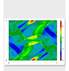
An MHD simulation of the Orzag Tang vortex (taken from this joint paper with Philppe Helluy). A new variant of the Lattice Boltzmann method is being used.
