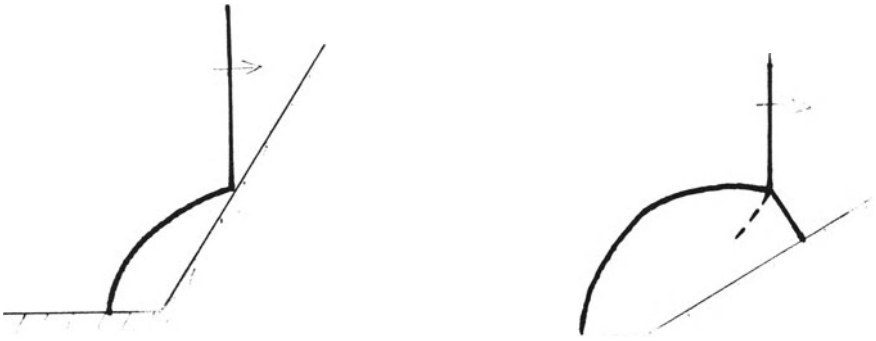
Fig. 4 A planar shock impinges onto a wedge, and, depending on the shock strength and wedge angle, give rise either to a regular reflection (left) or a Mach reflection (right). In the latter the reflected point has lifted off the wall to become a “triple point” from which a “Mach stem” connects to the wall.
