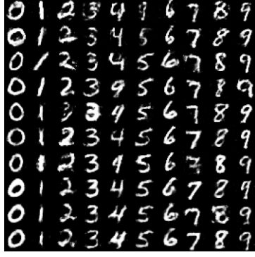
Figure 11: Outputs of model 9. Starting from standard dropout percentage of 0.5 at the top row, the dropout percentage is reduced 0.05 each row till 0.05 at the bottom row.
