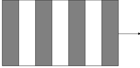
Figure 3. A two-phase rank-I laminate in two space dimensions with corresponding normal vector. The strains are constant in the shaded and in the unshaded regions. The volume fraction of both phases, 0.5 in the picture, is prescribed by the macroscopic parameter d .
